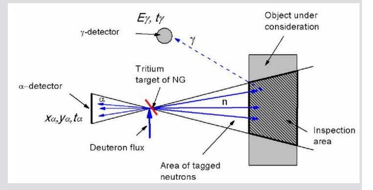
The energy and number of the gamma rays identifies the element from which it is emitted and essentially forms a "fingerprint" from which the element can always be identified.
