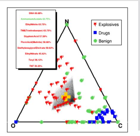
The RRTNIS system contains the inherent capability of being able to directly measure the amount of Carbon, Nitrogen and Oxygen present and identify conclusively the type of explosive or contraband drug. It makes it possible to scan a container on a volume element by volume element basis to uncover explosives, which are surrounded by inert substances.
